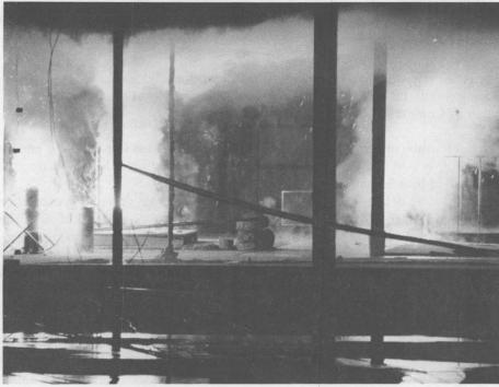
PHOTO AT LEFT shows fuel mixture burning around building support posts, about 40 seconds after ignition in the Seattle test fire. Note layer of hot smoke
